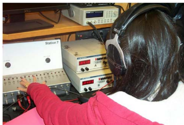
Figure 1. A Physical Systems student uses two sound sources and a mixing board to explore her perception of sound wave features, such as frequency and amplitude.
